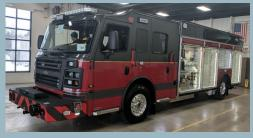
process of replacing two large fire apparatus (Engine 521 and Rescue 582) with one vehicle. This will provide crews with the simultaneous capability of suppressing fires while providing technical rescue services. Instituting this combined Engine / Rescue will reduce maintenance costs since the overall fleet size is being reduced.
