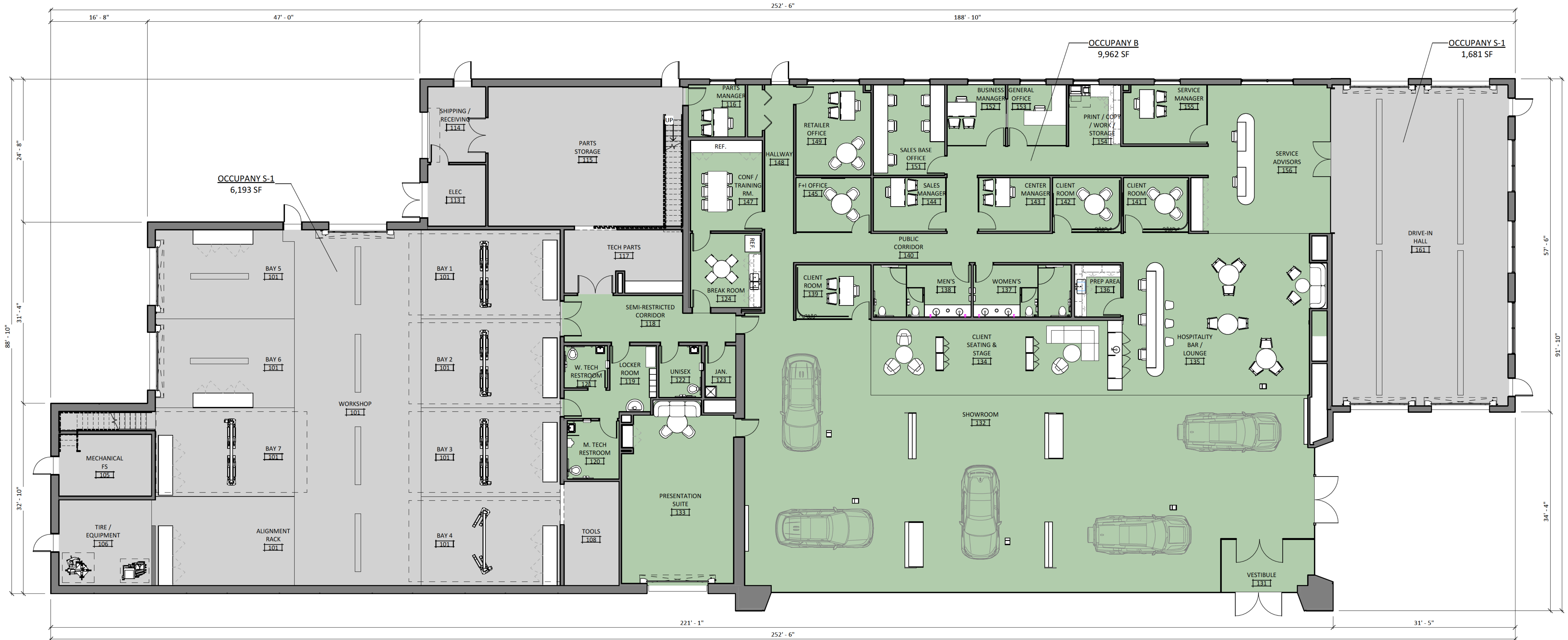
1 FIRST FLOOR AREA PLAN WITH OVERALL DIMENSIONS SCALE: 1/8" = 1'-0"
