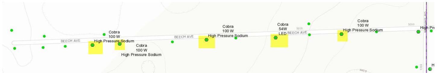
Green dots are existing power poles. Yellow highlights indicate existing streetlight locations of five (5) HPS fixtures.
